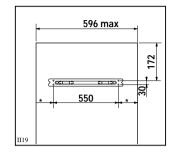
The panel must be fitted with a handle, as the dishwasher handle will be hidden by the panel.
